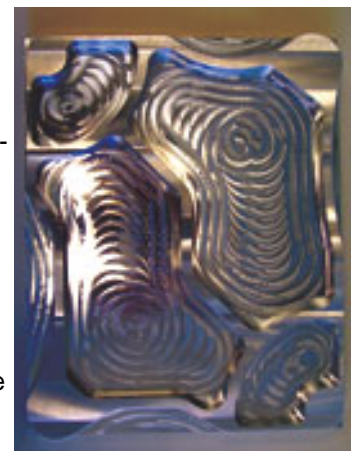
Note the corners in the conventional tool path (above) and the smoother TrueMill tool path (below).
