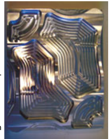
Note the corners in the conventional tool path (above) and the smoother TrueMill tool path (below).
